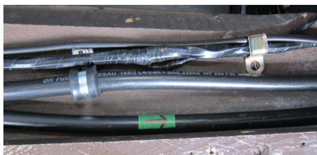
Fuel hoses on right side of the car
