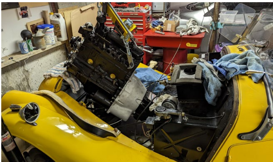
Gearbox mated to the engine and lowered into the car as a unit
