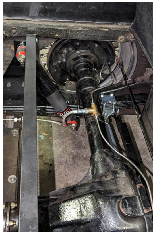
The five-leaf springs and Rutherford kit installed
